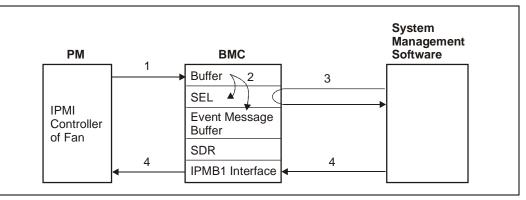
To make this possible the SDR of each sensor connected to an IPMI controller has to be written into the SDR repository of the BMC on the CPU board.
